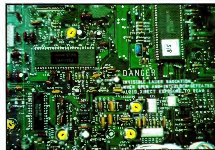
All the servo and laser adjustments and test points are available on one circuit board. The board can be accessed by removing the player's top cover.
